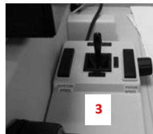
Motorized stage joystick and focus knob
